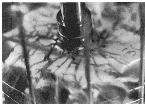
Fig. 14 Photograph of typical rotor failure
