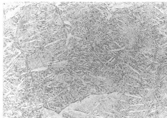
Fig. 4(C) Near HAZ, prior beta grains with fine acicular alpha-two martensite plates (1000 \times )
