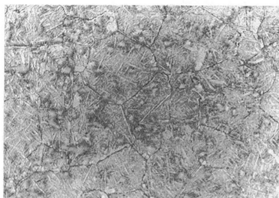
Fig. 2(C) Near HAZ, prior beta grains with fine acicular alpha-two martensite plates (1000 ×)
